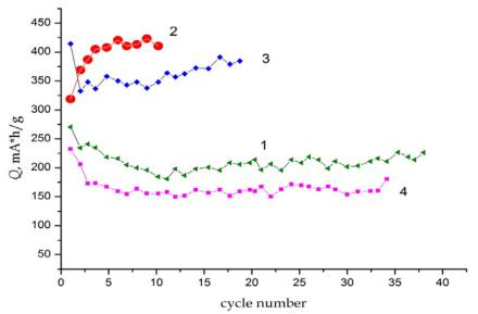
*Figure 2.* Specific discharge capacities vs. cycle number for synthetic graphite LBG-73 in perchlorate electrolyte:
