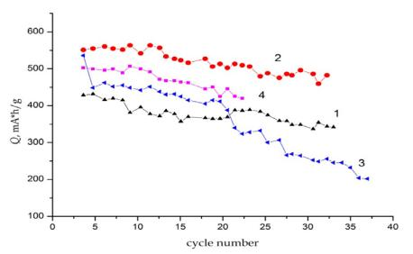
**Figure 4.** Specific discharge capacities vs. cycle number for synthetic graphite LBG-73 in hexafluorophosphate electrolyte: 1 – original, 2 – modified by monoaminoethanol, 3 – modified by diaminoethanol and 4 – modified by triaminoethanol pyrolysis products. Current load 10 mA/g
