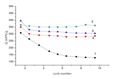
**Figure 3.** Specific discharge capacities vs. cycle number for natural graphite in hexafluorophosphate electrolyte: 1 – original, 2 – modified by monoaminoethanol, 3 – modified by diaminoethanol and 4 – modified by triaminoethanol pyrolysis products. Current load 10 mA/g
