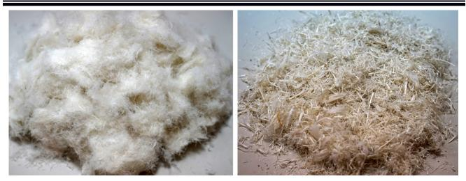
Fig. 1. Fibers which were obtained from chicken feathers (left) and separated rachis (right)
