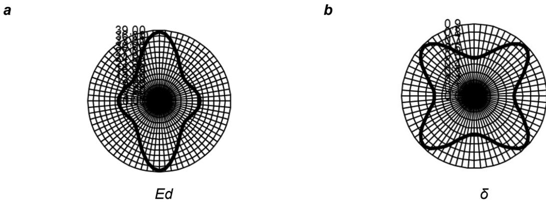
Fig. 4 Diagrams of indicators of (a) the modulus of elasticity  $E_d$  (MPa) and (b) the attenuation decrement  $\delta$  of the original materials with duplication parameters  $T_{v.p} = 150\text{ }^\circ\text{C}$ ,  $T_{n.p} = 100\text{ }^\circ\text{C}$ ,  $t = 15\text{ s}$ .
