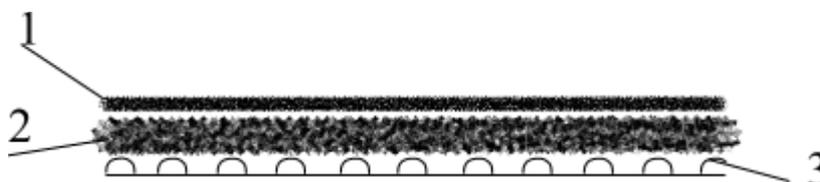
Fig. 2 Package with the content of nano-modified components in cross-section, 1 – non-woven material, 2 – low-melting components (polyethylene, polyester), 3 – upper material (suit fabric).
