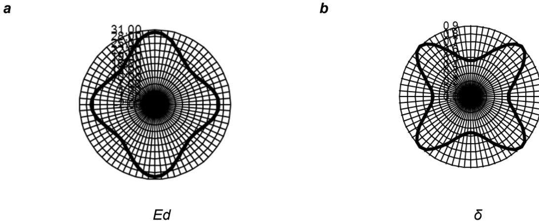
Fig. 3 Diagrams of indicators of (a) the modulus of elasticity  $E_d$  (MPa) and (b) the attenuation decrement  $\delta$  of the original materials with the duplication parameters  $T_{v.p} = 150\text{ }^\circ\text{C}$ ,  $T_{n.p} = 100\text{ }^\circ\text{C}$ ,  $t = 10\text{ s}$  ( $T_{v.p}$  and  $T_{n.p}$  – temperature of the upper and lower pads of the press).
