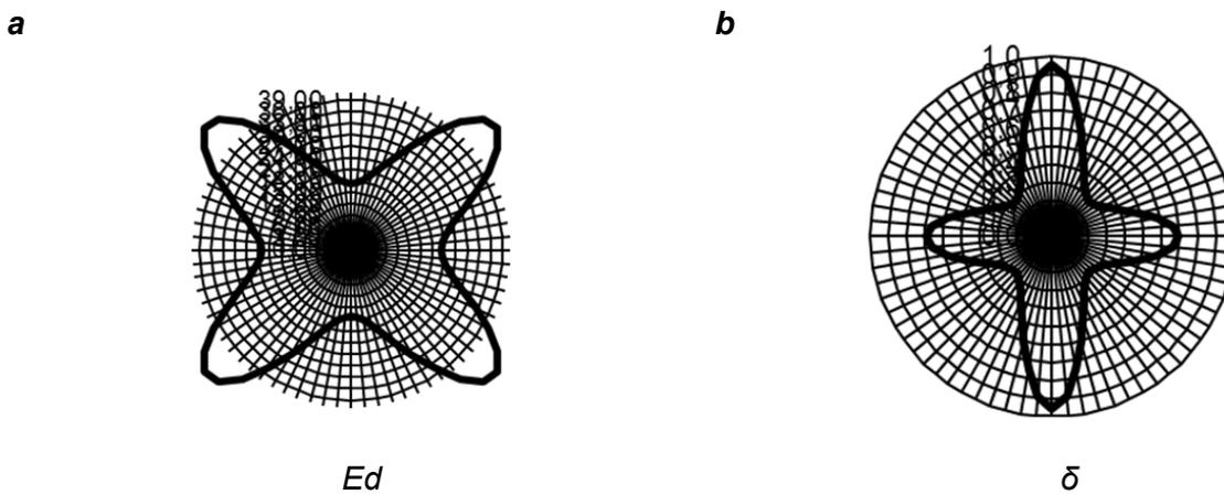
Fig. 7 Diagrams of indicators of (a) the modulus of elasticity  $E_d$  (MPa) and (b) the attenuation decrement  $\delta$  of the original materials with duplication parameters  $T_{v.p} = 160\text{ }^\circ\text{C}$ ,  $T_{n.p} = 100\text{ }^\circ\text{C}$ ,  $t = 15\text{ s}$ .
