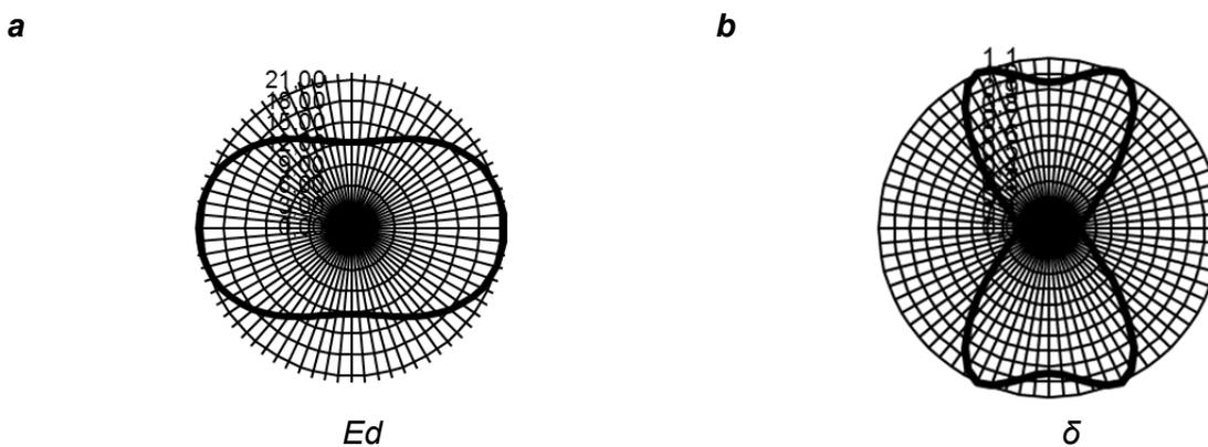
Fig. 5 Diagrams of indicators of (a) the modulus of elasticity  $E_d$  (MPa) and (b) the attenuation decrement  $\delta$  of the original materials with duplication parameters  $T_{v.p} = 150\text{ }^\circ\text{C}$ ,  $T_{n.p} = 100\text{ }^\circ\text{C}$ ,  $t = 20\text{ s}$ .
