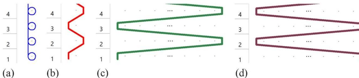
**Figure 1.** Lapping diagram: (a) first guide bar (pillar stitch), (b) third guide bar (elastomer thread), and (c) and (d) second and fourth guide bars (weft yarns).
