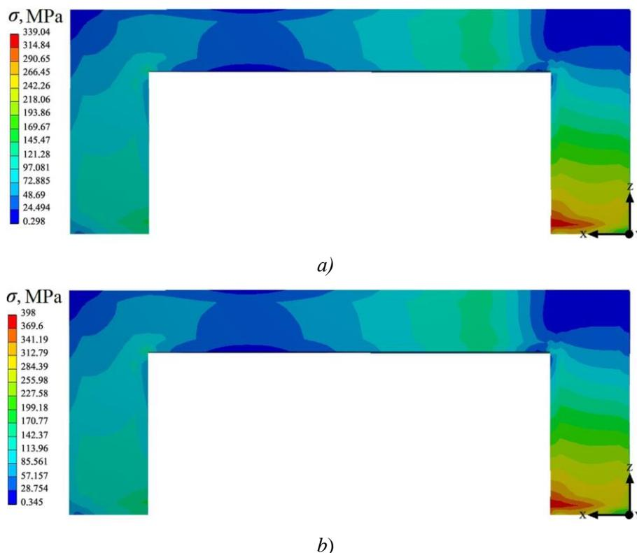
**Figure 3.** The distribution of the fields of stresses  $\sigma$  according to Mises in the flexible plate for cam at the following loadings: a)  $\bar{F}_{lif} = 14.03$  N and b)  $\bar{F}_{st} = 16.47$  N.
