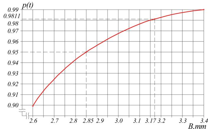
**Figure 5.** The dependence of probability of failure-free operation  $p(t)$  on the width of the console beam of the plate  $B$ .
