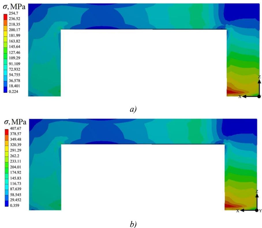
**Figure 2.** The distribution of the fields of stresses  $\sigma$  according to Mises in the flexible plate for the cam at the following loadings: a) mode 1 and b) mode 6, Table 1.
