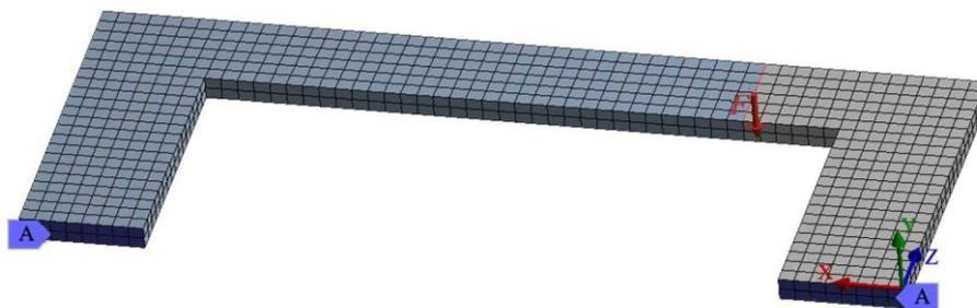
**Figure 1.** The model of the flexible plate for the cam according to the finite element method: *F* – force; *A* – areas of the hardcover of the plate.
