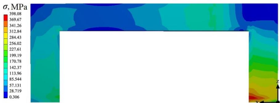
**Figure 4.** The distribution of the fields of stresses  $\sigma$  according to Mises in the flexible plate for cam at the loading  $\bar{F}_{lif} = 14.03$  N and the width of the console beam of the plate  $B = 3.17$  mm.
