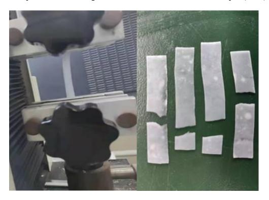
Figure 2.11 – PVA membrane mechanical test and after test
