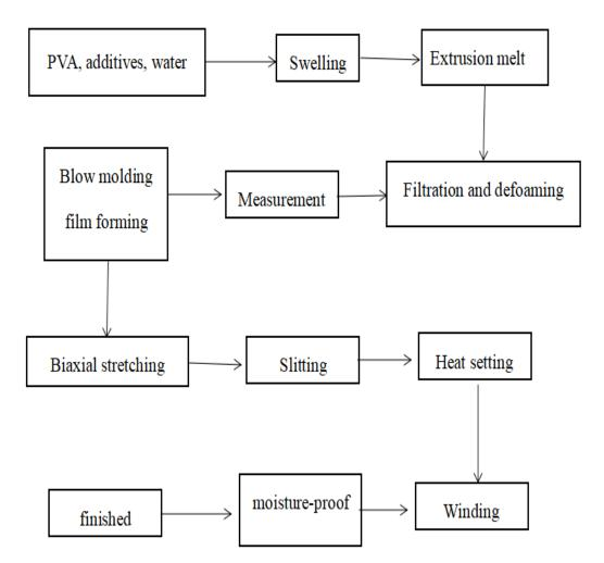
Figure 1.8 – Flow chart of wet extrusion blow moulding method
