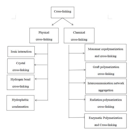
Figure 1.5 – The preparation methods of hydrogels
