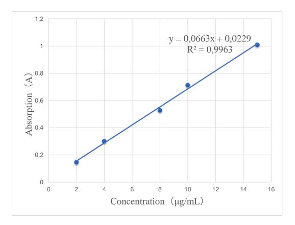
Figure 2.4 – Linear regression of absorbance at -192nm versus concentration
