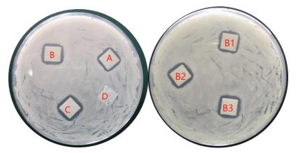
Figure 3.1 – Evaluation of the antibacterial effect of the hydrogel by the inhibition zone method
