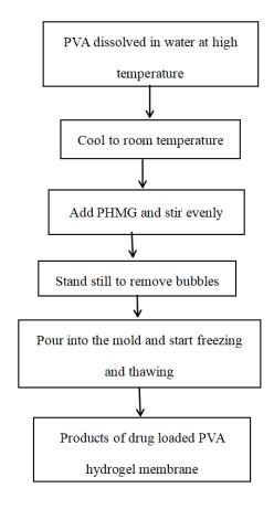
Figure 2.1 – Process flow chart for preparation of drug-loaded PVA hydrogel membrane
