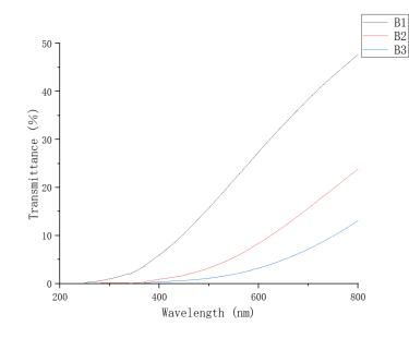
Figure 2.8 – Transmittance of PVA film with different freeze-thaw times and the same drug loading concentration
