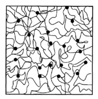
Figure 1.10 – Schematic diagram of PVA hydrogel after freezing and thawing
