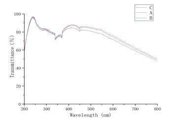
Figure 2.6 – Transmittance of PVA film with the same freeze-thaw times and
