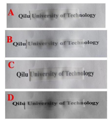
Figure 2.5 – The appearance of PVA membrane with the same freeze-thaw times
