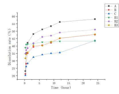
Figure 2.10 – Dissolution rate of drug-loaded PVA membrane at different times
