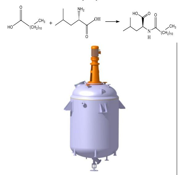
The upper part of the device with manhole, convenient observation and feeding. The purification equipment uses the following equipment with multiple glass observation holes for real-time observation of the extraction status, which is connected to the leucine-modified equipment through the main pipe.
