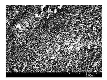
**Fig. 1.** FE-SEM image of ZnO layer obtained by anodization of Zn foil in a 1 M NaOH solution at 4 V for 30 min.
