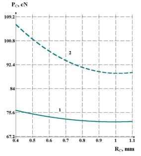
**Figure 9** Graphical dependencies (curves) reflecting influence of guide's radius on yarn tension after the guide for series C: 1 - for the polyethylene multifilament yarn 44 tex; 2 - for the polyamide multifilament yarn 58 tex
