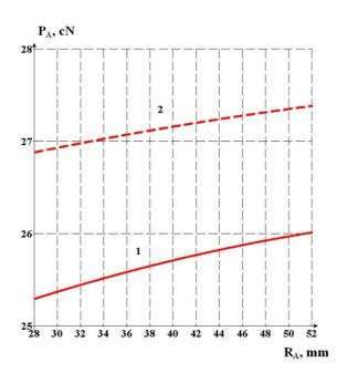
**Figure 7** Graphical dependencies (curves) reflecting influence of guide's radius on yarn tension after the guide for series A: 1 - for the polyethylene multifilament yarn 44 tex; 2 - for the polyamide multifilament yarn 58 tex
