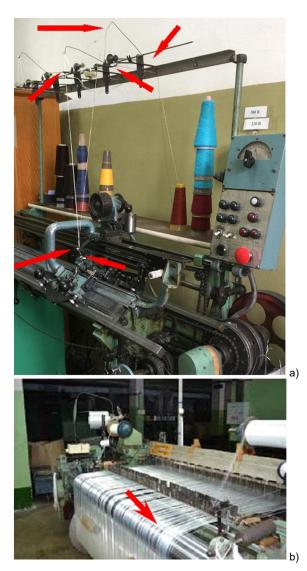
**Figure 2** Threading line in the knitting machine (a) and in the loom (b)
