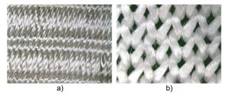
**Figure 1** Industrial fabrics and knits: (a) multilayer industrial fabric of polyamide multifilament yarns; (b) knit of polyethylene multifilament yarns
