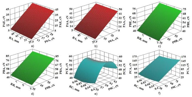
**Figure 6** Response surfaces for series A, B and C created to determine combined influence of the yarn tension before the guide and guide's radius on the yarn tension after the guide: for the polyethylene multifilament yarn 44 tex: a) series A, c) series B, e) series C; for the polyamide multifilament yarn 58 tex: b) series A, d) series B, f) series C
