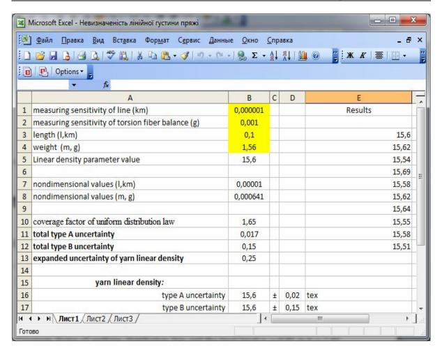
Figure 1. Calculation of measurement uncertainty of yarn linear density by using Microsoft Excel
