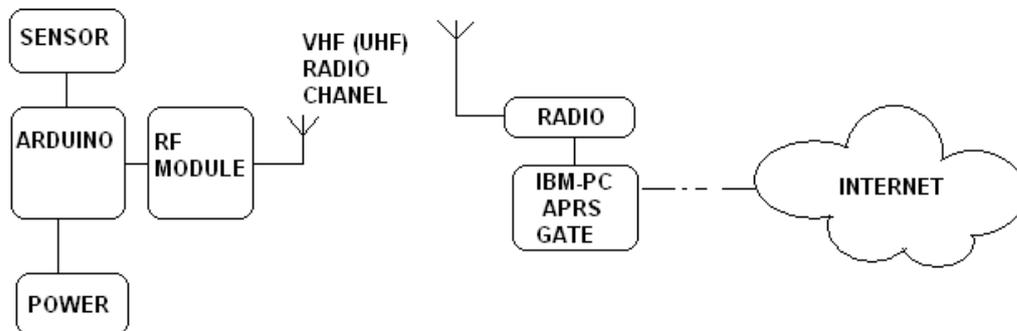
Figure 2 - Structural scheme of the system using the VHF radio network (range up to 100km)
